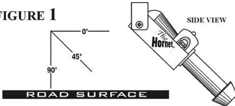
**Important:** The Hornet must have an unobstructed view of the road surface and be mounted in a forward direction at a 45° angle to the road surface, within a height of 6 inches to 3 feet to achieve maximum effectiveness.
